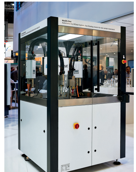
Fig. 1. The new plasma treatment unit is highly compact as it no longer requires a 6-axis robot or additional linear axes © Plasmacore, Jan Dufelsiek
