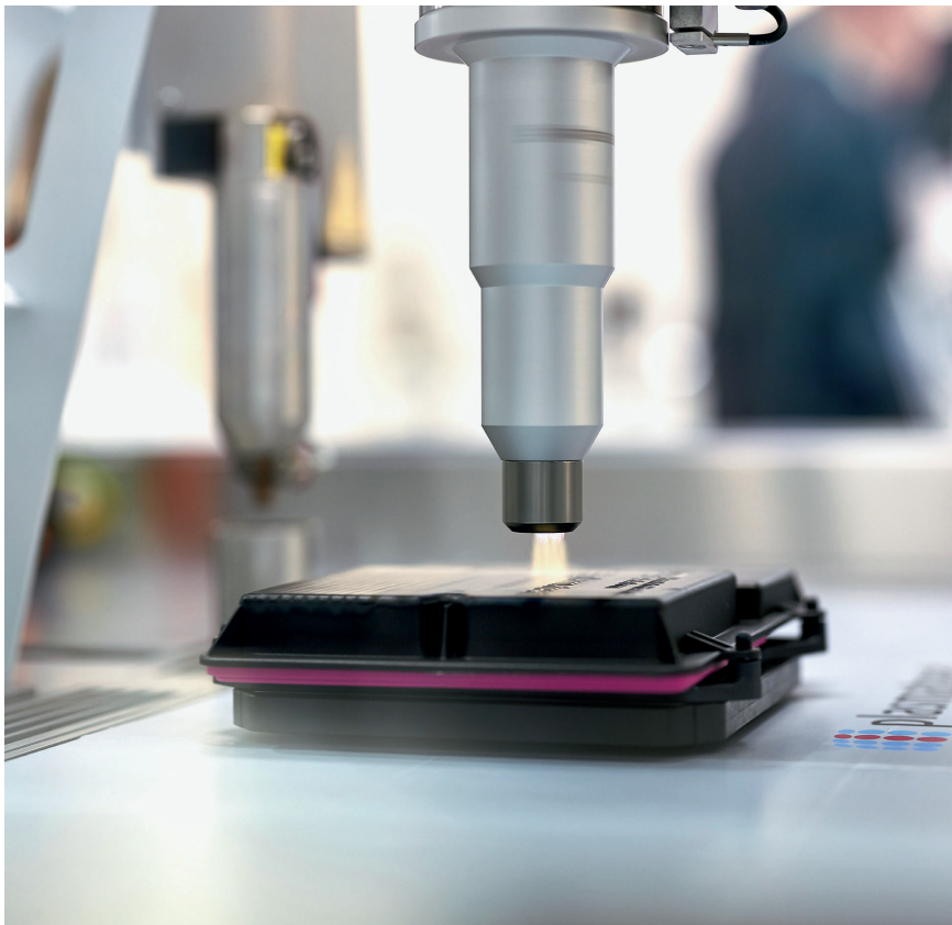
A floating planar mover carries the workpiece exactly into position for surface treatment
